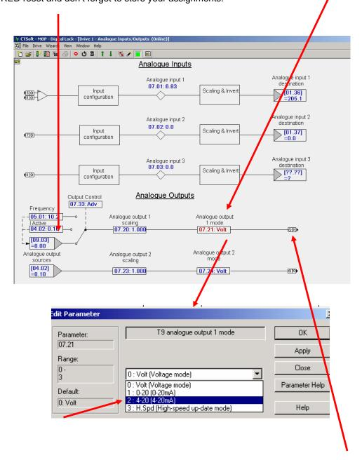
This would complete this scenario with pin 9 providing a Ramped 4-20mA output signal under control of Increase/Decrease Operator pushbuttons.
