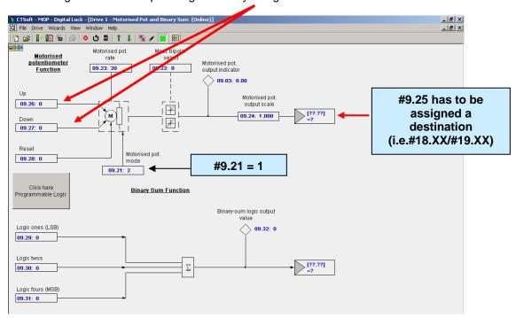
Parameter #9.03 should tumble between 0 and 100.0 and cover this span in 20 seconds per #9.23.
