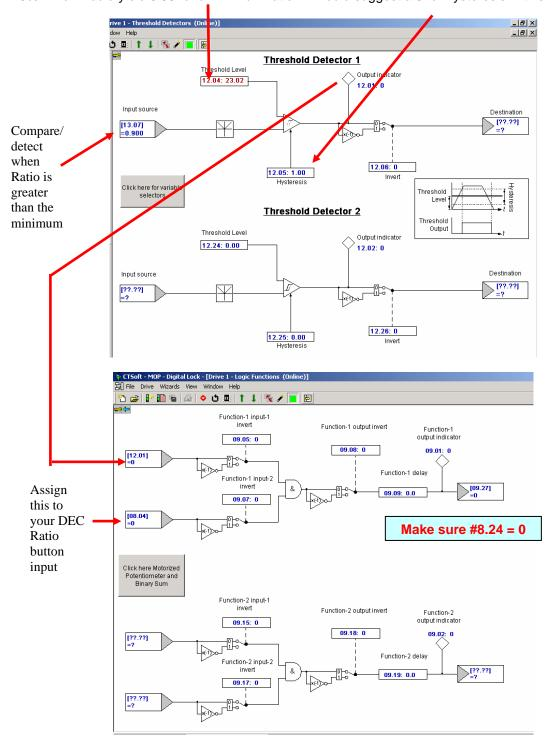
Depress RED reset to make you assignments take effect. One can check the operation by observing #13.07 while depressing the newly assigned INC/DEC buttons. The rate of Ratio change can be altered by parameter #9.23. Depress RED reset and don't forget to store your assignments.
