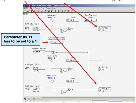
One can check the operation of these inputs now by depressing the RED reset button on the front of the UnidriveSP and observing #9.03 while depressing the newly assigned INC/DEC buttons.
