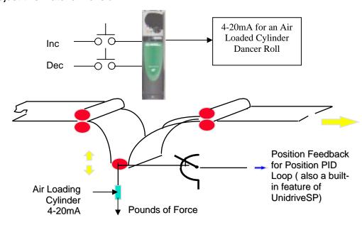
First we must assign 2 inputs as the Increase and Decrease function. In this example, I've selected Input 4 and Input 6 respectively (pins 27 and 29 respectively). Mapping Input 6 to the MOP Increase (parameter #9.26) and Input 4 to Decrease (#9.27) will accomplish this mapping.
